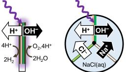
**Figure 2.** Proposed applications for photoaciddye-modified bipolar membranes of light-driven redox chemistry and desalination of salt water.
