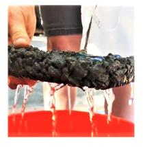
We also did a side-by-side demo showing how flooding looks with normal concrete compared with pervious concrete. Many people walking by took a moment to see the demo, and learn about the 1:1 ratio each ton of cement releases of CO<sub>2</sub>. Many people were shocked to learn this fact along with others, and were wildly surprised by how the water went right through the pervious concrete!
